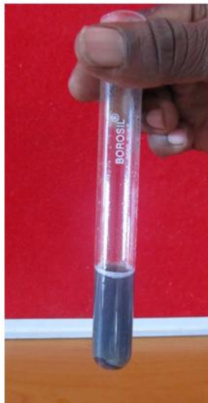
Development of violet colour on adding \text{CuSO}_4 & \text{NaOH}
